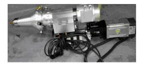
\* Head mounted on motion system – the linear guider and the servo motor
